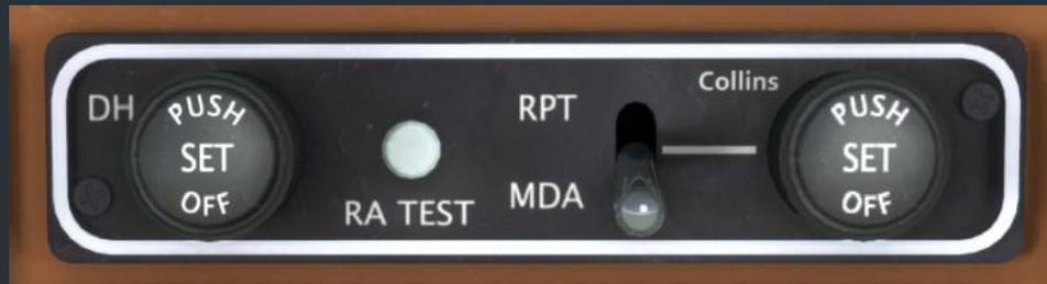
The right knob is used to set either a minimum descent altitude, or reporting altitude. The small switch to the left of this knob is used to select which of these two altitude alert modes is active. Pressing the center of the knob will hide either altitude and alert from the PFD display.
