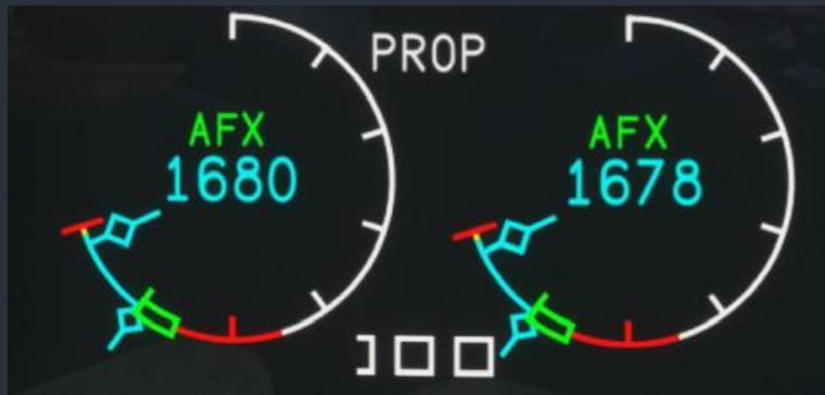
NOTE: Also within the RPM scale, an optional “BETA” text may appear when the power levers are within the beta range. This feature is enabled by default, but may be disabled with the “Beta Annunciator” persistent option on the tablet options page.
