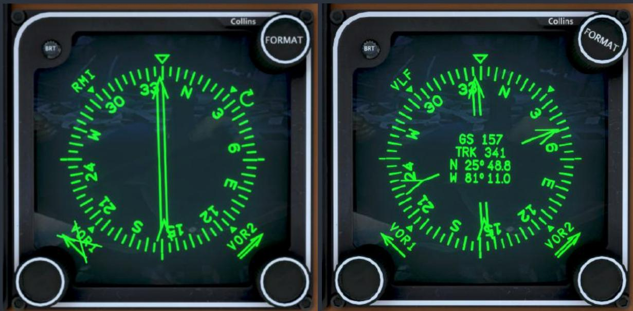
VLF mode displays the same information as RMI mode, except the centers of the two needles are removed and replaced with the Flight Management System's (FMS) position estimation information. This includes ground speed, ground track, longitude, and latitude, or "VLF FAIL" if the VLF/Omega navigation system is disabled.
