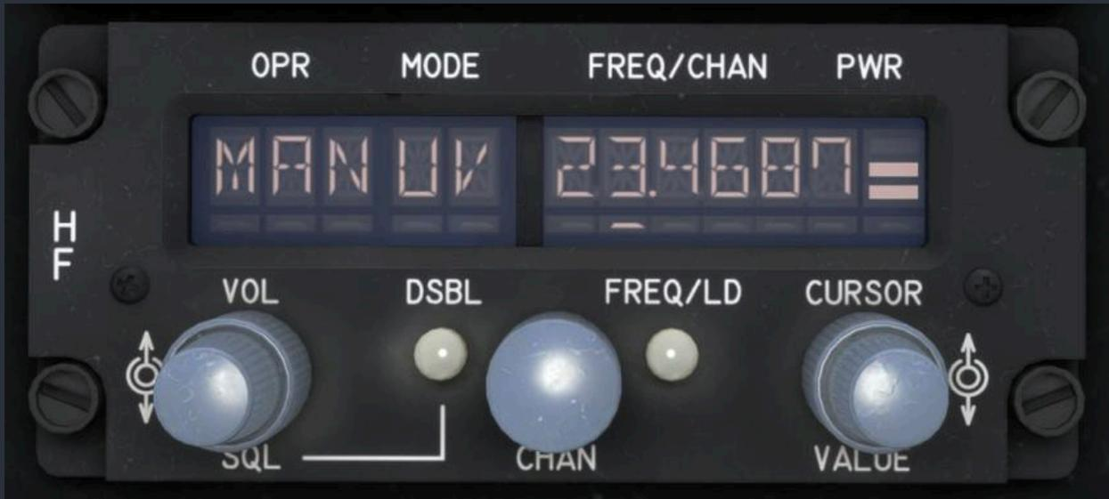
NOTE: For the HF radio to be audible, the “HF” audio switch on the pilot’s audio control panel must be in the up position.
