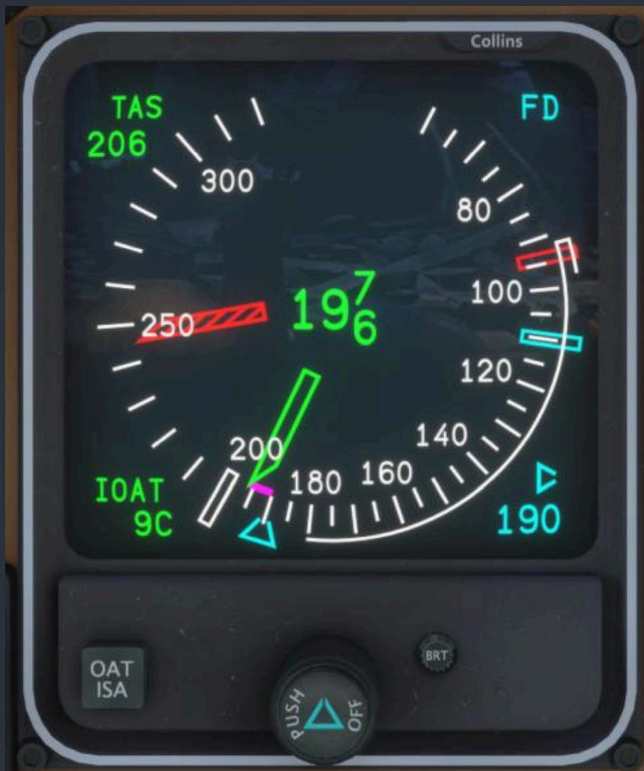
The outside of the airspeed scale is adorned with the customary red line to indicate the single engine minimum controllability speed (V<sub>mc</sub>), and a cyan line to indicate the best single engine rate of climb speed (V<sub>yse</sub>). A single white arc denotes the flap operating range, and a double white arc denotes the flaps extended stalling speed. A white rectangle marking at 200 kts indicates the maximum landing gear extension speed.
