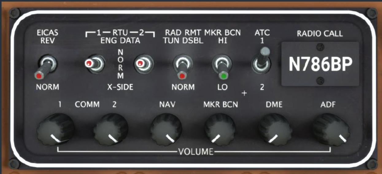
NOTE: All reversionary mode switches possess an integrated red/orange LED in the switch lever, which illuminates when the switch is positioned in a reversionary mode.
