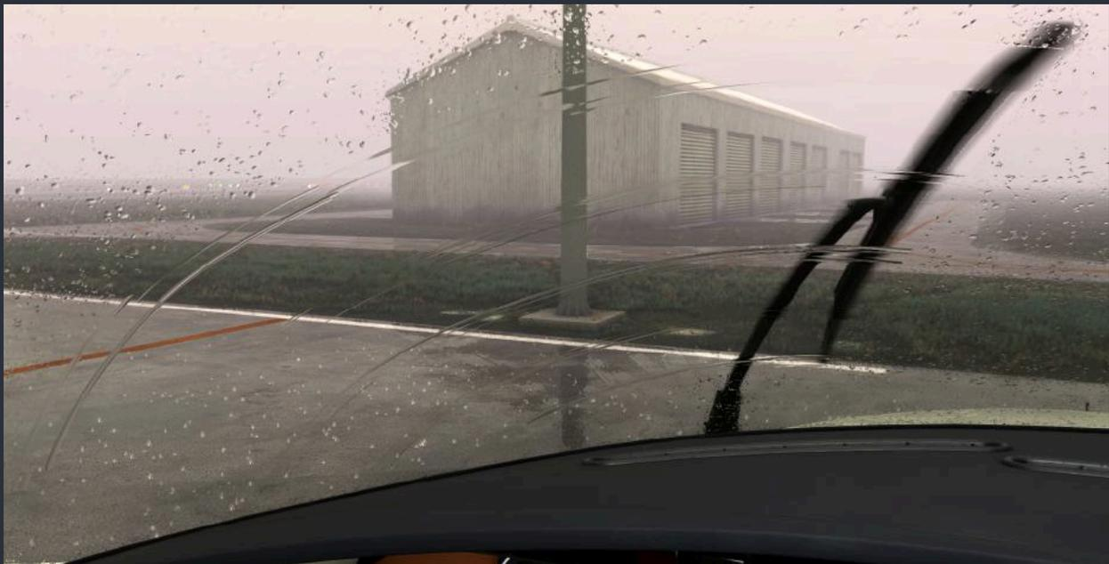
NOTE: The wipers can cause a slight performance degradation (1 fps), **only when they are operating**. The wiper effects can be removed completely by making a small edit to the behaviors XML file in the root aircraft folder. In "Starship\_Interior.XML", search for "WindshieldWiperEffects", and follow the instructions to make this simple change.
