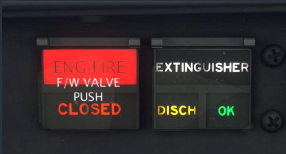
The fire detectors and extinguishers can be tested by pressing the “FIRE DET” and “FIRE EXT” buttons on the pilot’s left subpanel. When the “FIRE DET” button is pressed, the “ENG FIRE” annunciator should illuminate and trigger a master warning. When the “FIRE EXT” button is pressed, the green extinguisher “OK” annunciator should illuminate. The fire bottle charges can be refilled from the Engine Visualizer pages of the tablet interface.
