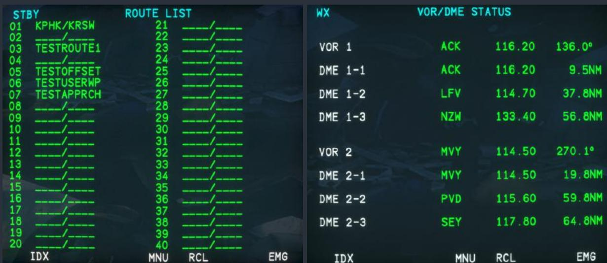
The VOR/DME Status screen shows the current frequency, received identifier, and DME distance to all six DME receivers and two VOR receivers on the aircraft. This screen is useful for monitoring the automatic navaid tuning required to generate an accurate positional estimate when GNSS is deselected as a source of position information.
