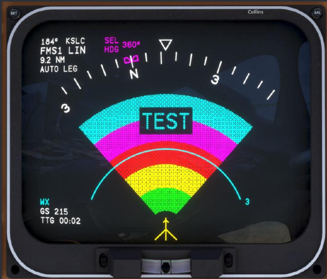
Radar test pattern on ND ARC display
