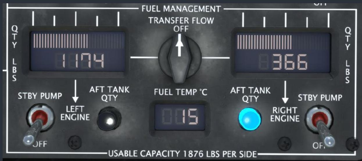
NOTE: DO NOT mistakenly add the normally displayed TOTAL quantity with the aft tank quantity to arrive at the total fuel aboard, as this will overestimate the total quantity of fuel remaining. The normally displayed value is the total quantity in BOTH main and aft tanks.
