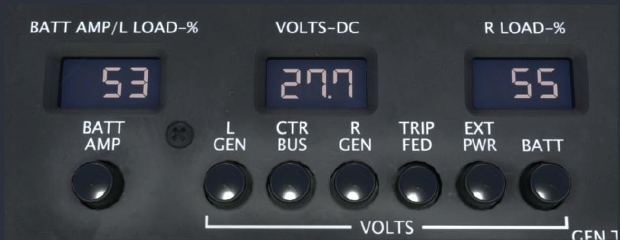
The voltmeter screen in the center of the panel displays the voltage at any one of the six sensing locations, selected with the radio push buttons below the screens. Refer to the “Overview Electrical Schematic” in this manual for a graphical depiction of each of these sensing locations, and take note of the diodes that may produce different voltages across the system when all bus ties are closed.
