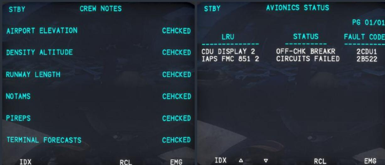
The Avionics Status screen displays any currently active fault codes from any of the aircraft's Line Replaceable Units (LRU), and decodes them into human readable status messages. For example, if the copilot's side Sensor Display Unit (SDU) has overheated, the status message "SENSOR DSPLY 2 OVERHEAT" will be displayed. Crew notes are accessed from the Index screen, and can contain any items programmed through the Data Base Unit (DBU).
