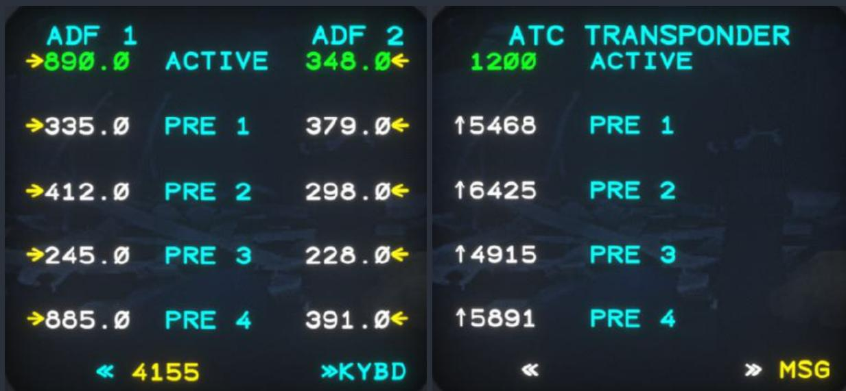
NOTE: To enter ADF frequencies with decimal components (usually 500 Hz spacing), the numerical entry MUST consist of five digits with a leading zero, if the frequency to be tuned is less than 1 MHz. For example, an entry of "07455" will tune a frequency of 745.5 kHz.
