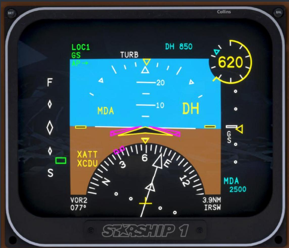
To the left of the artificial horizon, a speed deviation indicator will be displayed any time the speed reference bug is displayed on the on-side ASI. A green rectangle will move vertically to indicate whether the indicated airspeed is higher or lower than the reference airspeed. Full deflection of the indicator represents a deviation of 10 kts. In the event of an on-side Air Data Computers (ADC) failure, the speed deviation indicator is replaced by a red “SPD” flag.
