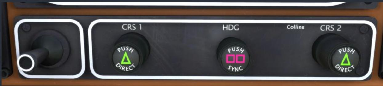
The heading rotary knob is used to adjust the heading reference bug for whichever Flight Control Computer (FCC) is currently selected as the autopilot source with the "AP XFER" button on the Autopilot Panel (APP). Pressing the center of the knob will synchronize the heading reference with the aircraft's current magnetic heading.
