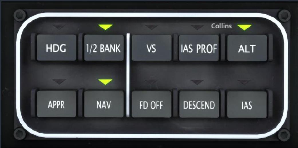
In Descend mode, the FCC will continuously command a reference airspeed 25kts below the barber-pole speed (Vmo) until reaching 10,000 feet, at which point the reference speed will become steady at 225 kts. If the reference speed is adjusted manually using the airspeed reference knob on the ASI while Descend mode is activated, then the new speed offset with Vmo will be maintained until 10,000 feet.
