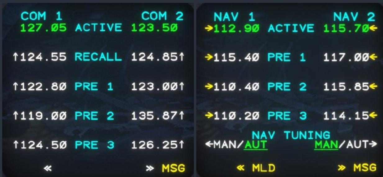
NOTE: The COM screen of the CDU supports 8.33 kHz frequency tuning, a feature unsupported by the actual hardware. While these frequencies cannot be displayed by the RTU's, they can be adjusted with the knobs, and will be displayed on the CDU COM screen.
