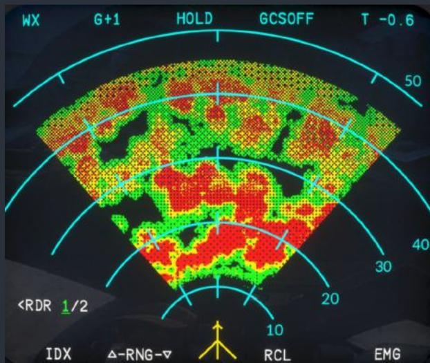
The Radar screen depicts the weather or terrain radar buffered image with the aircraft symbol at the bottom of the display. All radar parameters are controlled via the Radar Control screens on the Control Display Unit (CDU) and the CDU keypad, except range, which can be adjusted with the up and down line select keys on the MFD. The bottommost left line select key on this
